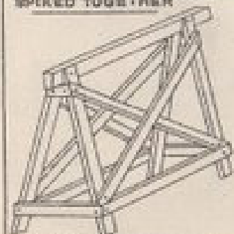
Fig. 5. FOUR LEGGED TRESTLE OF RECTANGULAR TIMBER SPIKED TOGETHER
